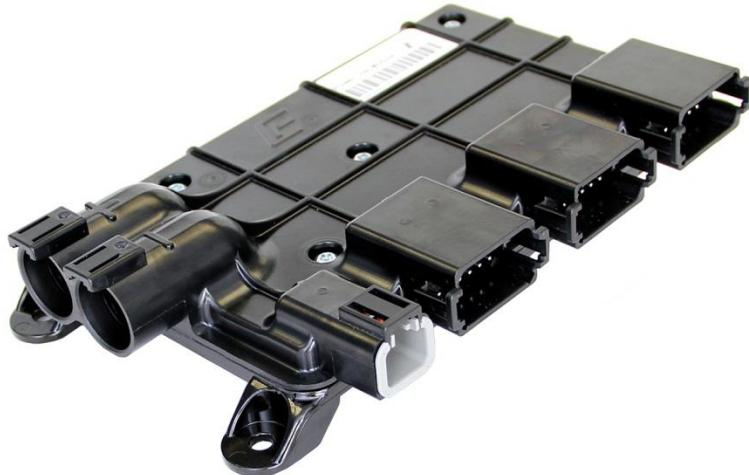
Each of the 12 PDM outputs can switch or proportionally drive 15A loads and feature built-in over-current detection and shutdown capability. Outputs can be paired to run up to six electric motors with H-bridge direction control.
