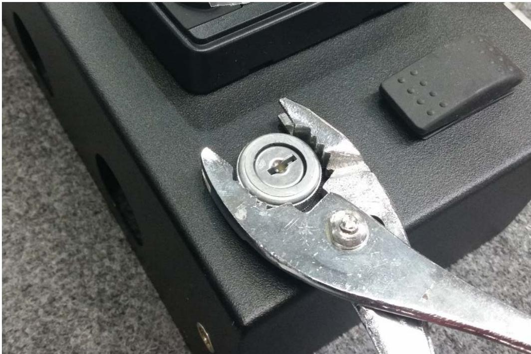
The key switch is properly installed from a mechanical point of view when:
