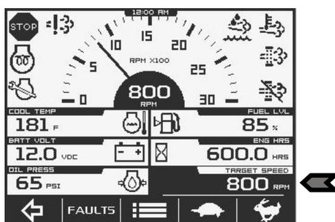
**NOTE:** Target Speed gauge appears for 5 seconds when the user throttles the engine (see arrow above)
