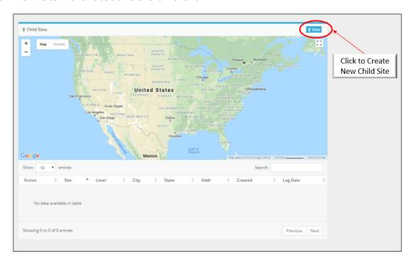
Once the New Child Site button is clicked, a new window will open to fill out a form for the child site similar to the form for the original site setup. Once the information is all entered, click the Save Site button to save the site under the original company site.
