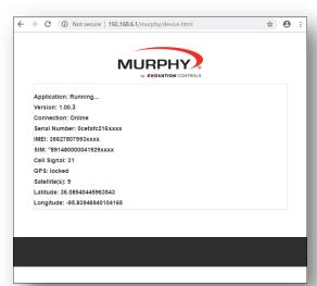
Application: States whether the application is running or not running. This should be running at this stage
