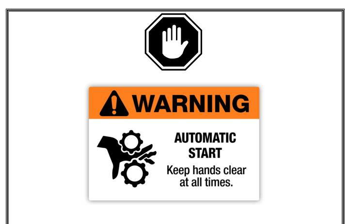
The CONNECT device can be used for remotely starting an engine when used in conjunction with Murphy's PowerCore<sup>®</sup> controllers and start unexpectedly. Please be cognizant at all times of hands and other objects that are in close proximity to the machine(s) being controlled as they may commence operation suddenly and without warning
