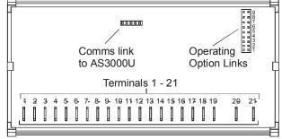
The links must be set correctly before the AS3000 is connected or used.
