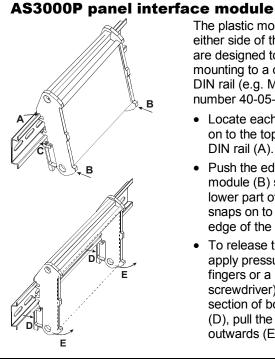
The plastic mouldings on either side of the AS3000P are designed to allow snapmounting to a control panel DIN rail (e.g. Murphy part number 40-05-0474):-
