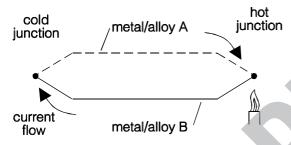
If the 'cold' junction is disconnected, this potential for current flow can be measured as a milli-voltage ( $V_{tc}$ ) between the two disconnected wires:—
