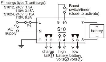
1 Relay de-energises (contacts close) on fault 2 Relay energises (contacts close) on fault
