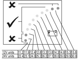
ESI accuracy is ±0.3V for 12V units, ±0.5V for 24V units.
