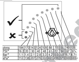
\* pressures above are theoretical values calculated from typical sender performance. ESI accuracy is ± 5.7 PSI at primary (fault) point (20PSI) and ± 15PSI for the rest of the scale. Actual in-service accuracy will be affected by sender tolerance and connecting wire resistance.
