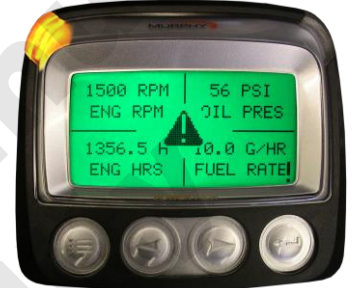
4-up display with warning fault
