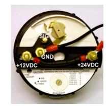
3) Add a terminal nut (supplied with 20.70.0176) to the GND (0V) stud, screwing down the nut to be flush with the panel securing clamp.
