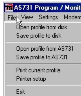
The **File** menu includes options for managing AS731/732 program profiles, including opening from and saving to disk, uploading to and downloading from the Autostart, and for printing.
