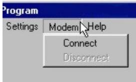
The **Modem** menu options are only available when the PC is fitted with a modem. These options allow the user to connect and disconnect a communications link with a remote Autostart.
