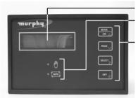
LED indicators: Auto (green), Manual (amber) Operator control keys:-On/mode: turns on unit and allows selection of auto or manual modes Page: used for scrolling of display information Select: used during program mode Off: powers down the unit, stops the engine and resets a fault condition.
