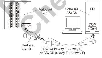
The software is used to create and edit program 'profiles', which can be downloaded to the Autostart over the communication link, quickly and error free.
