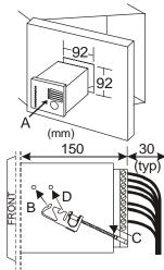
The AS705 is mounted in the front of a control panel through a DIN standard aperture, 92 mm  $(3^{5/8})$  square.
