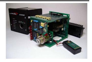
Remove the Autostart circuit board assembly out of the back of the unit. The top side covering plate may need to be raised slightly so that it clears switches 1 – 5 on the top circuit board.
