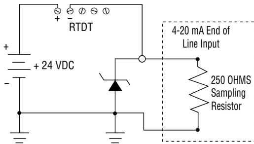
plied by the operating current. A transmitter with 24 volts at its terminal and with maximum current (30 mA for an open RTD) will dissipate 0.7 watts of power. This can be significant if the RTD sensor can be affected by thermal gradients from the transmitter.
