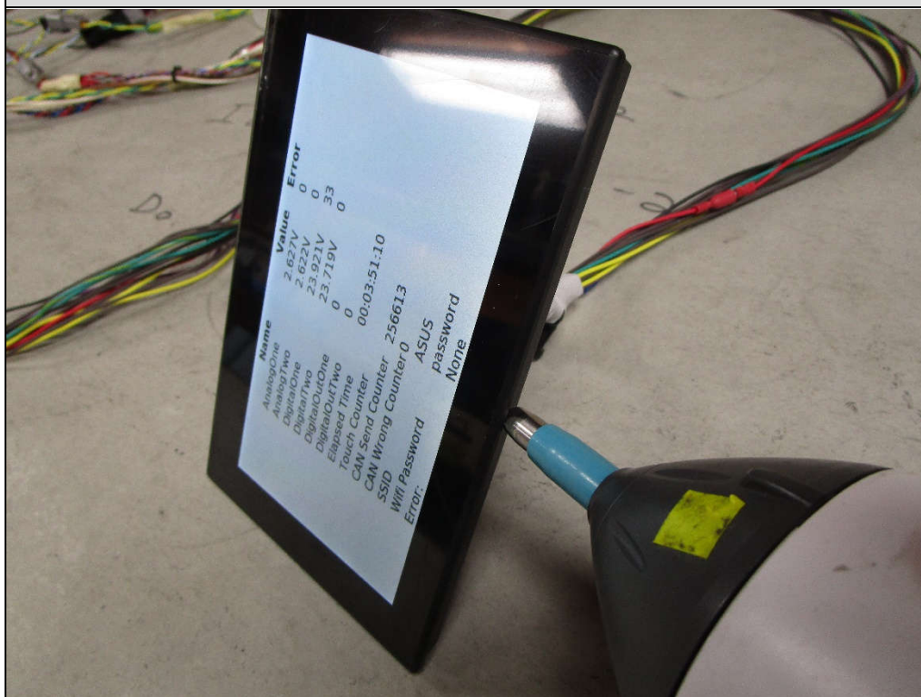
Test Setup for Electrostatic Discharge (ESD)
