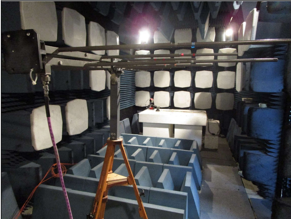
Test Setup for Radiated Immunity: 80MHz to 1GHz, Horizontal Polarization
