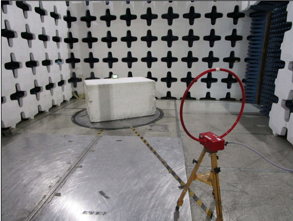
Test Setup for Radiated Emissions: 150kHz to 30MHz, X-axis Polarization
