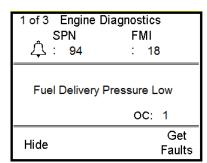
Use the **Left** and **Right** arrows to scroll through the screens if there is more than one stored fault. Each saved code shows the SPN (Suspect Parameter Number), FMI (Failure Mode Identifier), and OC (Occurrence Count). The OC indicates if the same fault occurred more than once.
