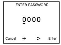
**ENTER PASSWORD** screen – Enter the four-digit value in the spaces provided. Start at the furthest left value and use the **Left Arrow** to increment the number and the **Right Arrow** to move to the next position. If you do not have the password, contact the OEM from whom the engine was purchased. For more information, see **OEM Menu Options** on page 9.
