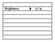
The other menu items disappear and Brightness remains. Use the **Left** and **Right Arrow** keys to increase or decrease the backlight intensity of the display in 5% increments.
