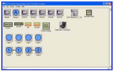
This first part of the software suit allows the user to choose the module or modules being used and to configure the I/O as required for the application. This process is as simple as looking for the HCT product on the drop down menu and placing it onto the open screen.
