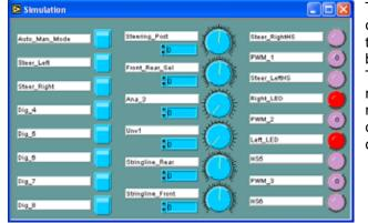
The last part of the Intella suite is intended to promote safe operation and allows the user to simulate and de-bug the code so that the majority of any obvious errors can be found and corrected before installation onto the actual equipment.
