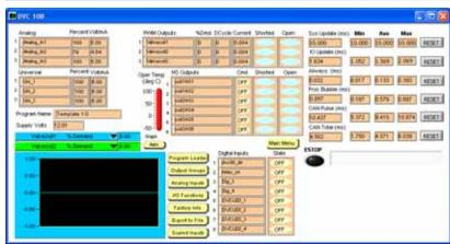
The **Program Loader Monitor ( PLM )** gives the user the opportunity to not only modify and upload the completed application code to the controllers but is also used to update the BIOS and other related software for the DVC series.
