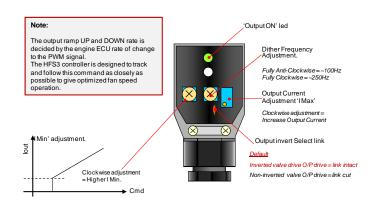
View of HFS 3-12V with lid removed and no cable shown for clarity
