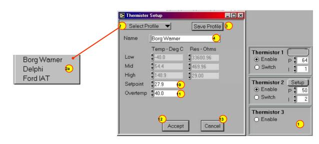
The HFS software includes several pre-characterized thermistor calibration profiles. These are accessed by pressing <Unit Settings>, <Setup> (for the thermistor to be calibrated), <Select Profile>. This allows selecting one of these thermistors from a drop down list.
