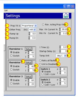
Set the Maximum valve current here from 0 – 100%. Maximum current (100%) depends on coil Ohmic value and supply voltage and will determine the fans maximum speed.
