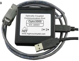
The optical communications also allows high speed data transfer between the host PC / laptop and the controller for real time diagnostics and fast set-up or programming.
