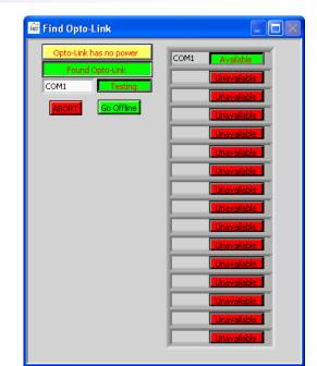
The Opto 3000 should be connected to the host PC first and the HFS software started. The PC will immediately check the available ports, display a list ( shown right ) of available serial ports, find the Opto 3000 and connect. If the Opto 3000 is connected to an HFS that has power applied, the program will take a few seconds to check module validity and then display the settings from that module. At this point, the user may enter a password if changes to settings are required.
