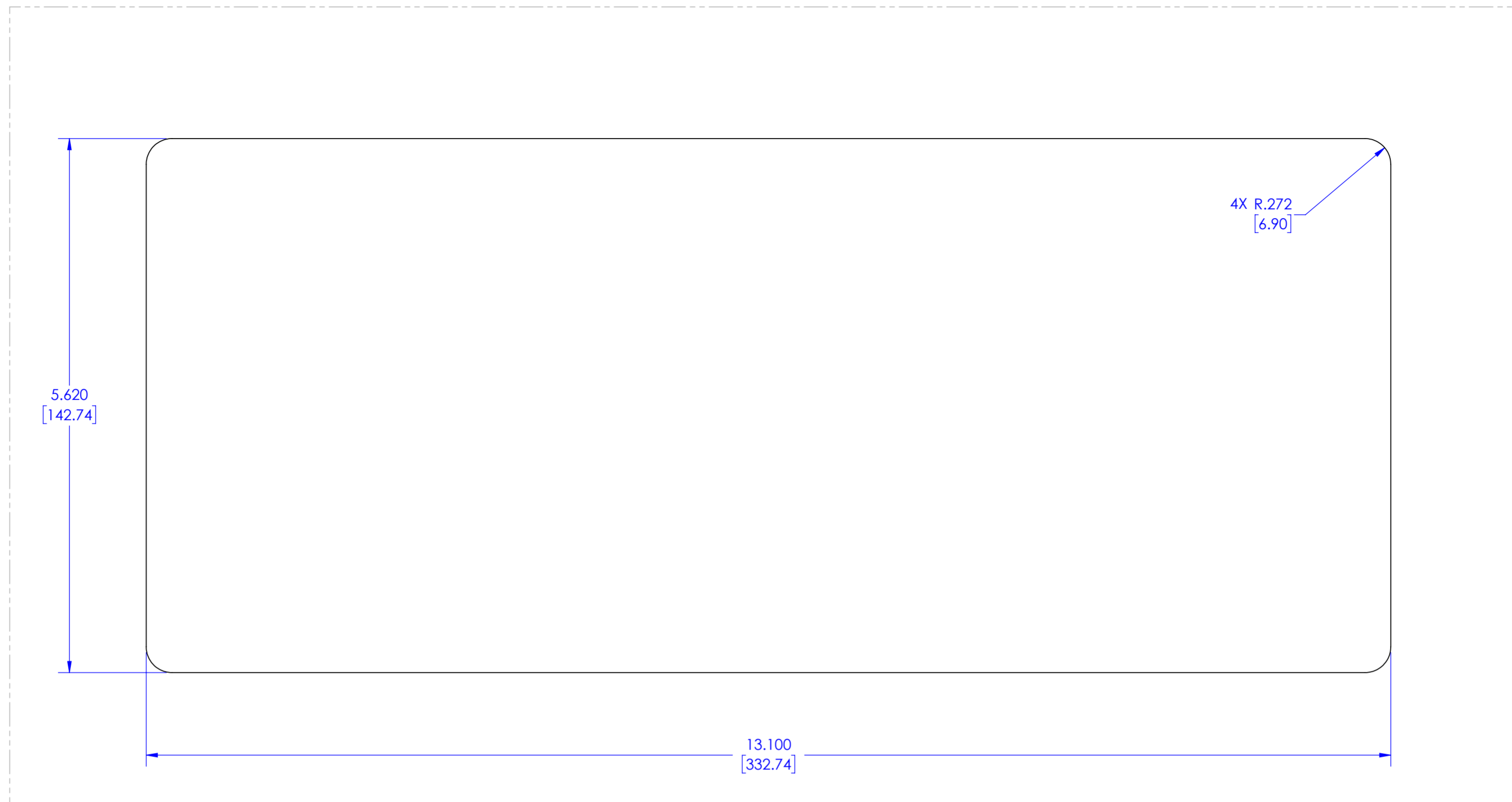
RECESSED MOUNT PANEL CUTOUT DIMENSIONS FULL SCALE
