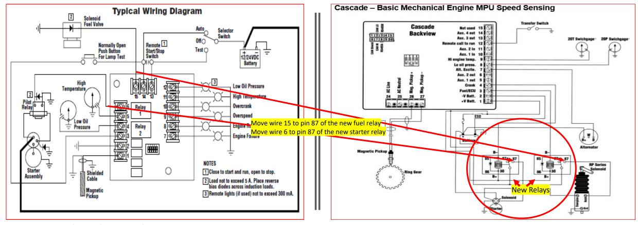
Outputs to the Relays on the ASM150 are B+
