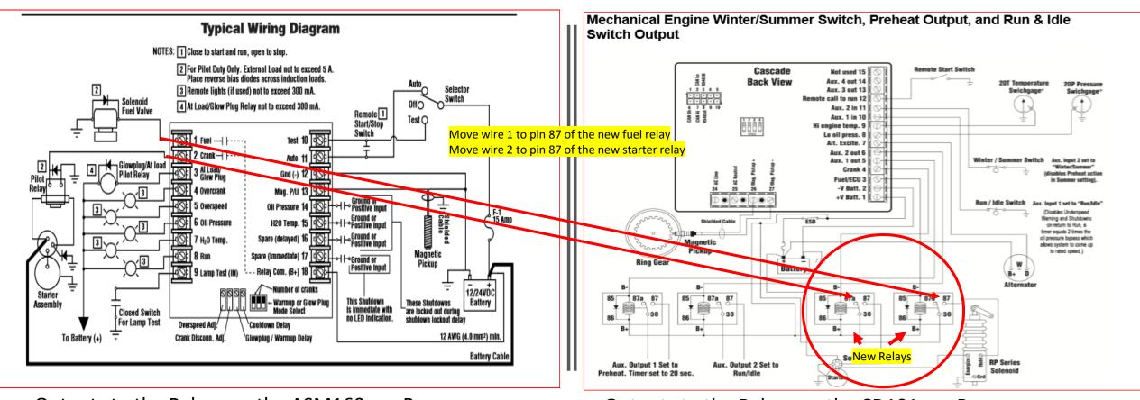
Outputs to the Relays on the ASM160 are B+
