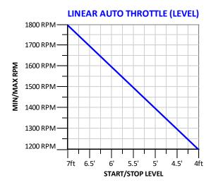
**NOTE:** In order for linear auto throttle to work correctly the auto start/stop function and auto throttle method need to be set to the same transducer type.
