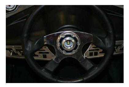
i. Hint: Be sure to keep the steering wheel in a horizontal position when you remove it as an aide to reinstalling it with proper orientation.
