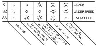
Nominal speed calibration and relay trip levels are set via four multi-turn potentiometers – see Calibration section overleaf. The 3ST also features a meter output, which may be used for calibration and/or engine speed indication.
