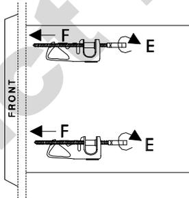
Microstart extends to 215mm behind the panel front; an extra 30mm should typically be allowed for the connection of a wiring loom.
