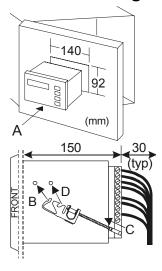
The AS730 is mounted in the front of a control panel through a DIN standard aperture, 140mm (5½") wide by 92mm (35/8") tall.
