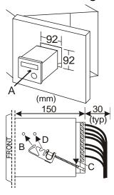
The AS710 is mounted in the front of a control panel through a DIN standard aperture, 92 mm (3<sup>5</sup>/<sub>8</sub>") square.
