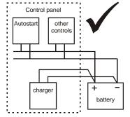
External Slave Relays are a recommended connection on all outputs (as shown right), either to achieve the required load switching capability, or to reduce wear and tear on internal relay contacts.
