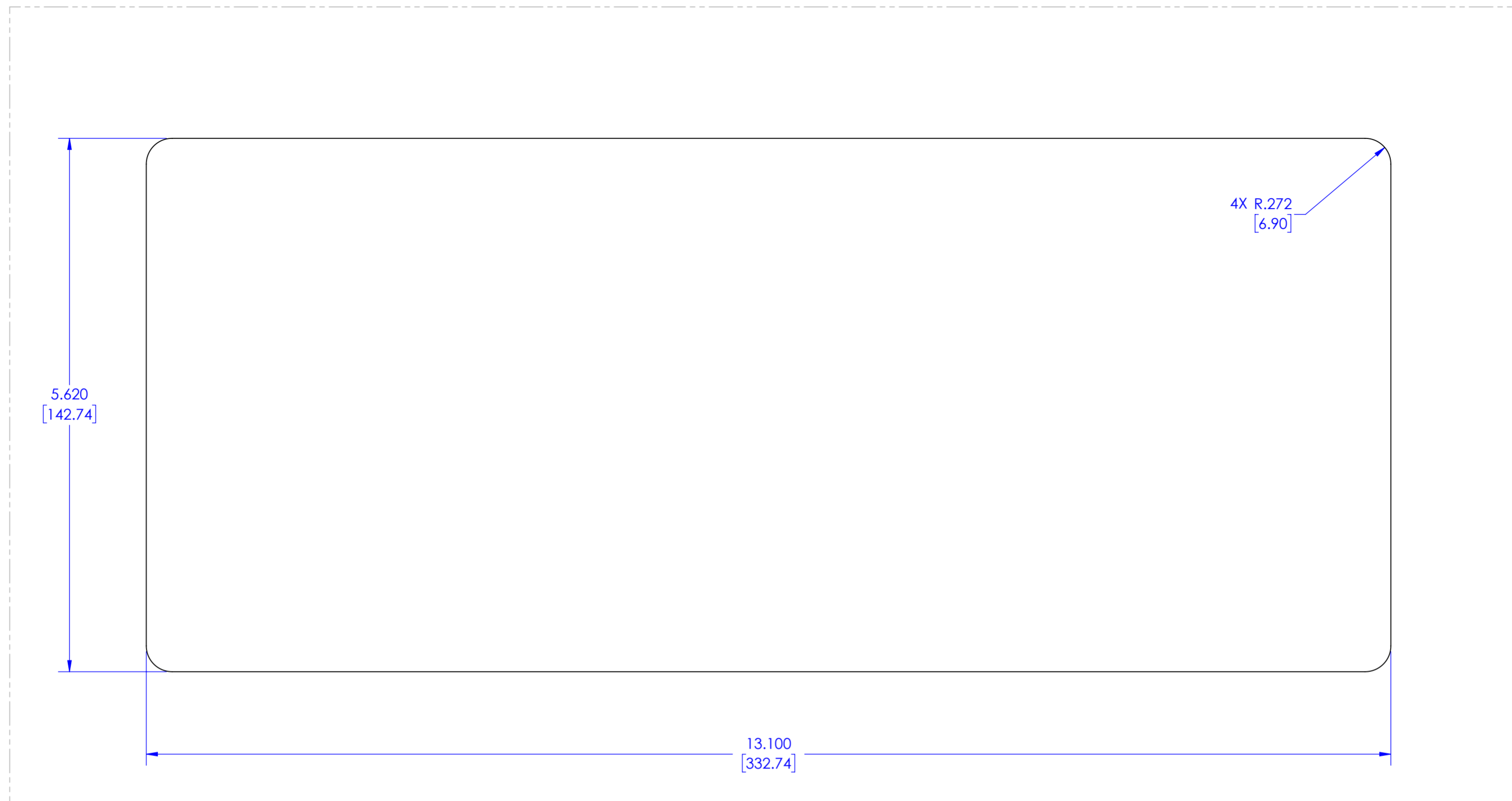
RECESSED MOUNT PANEL CUTOUT DIMENSIONS FULL SCALE
