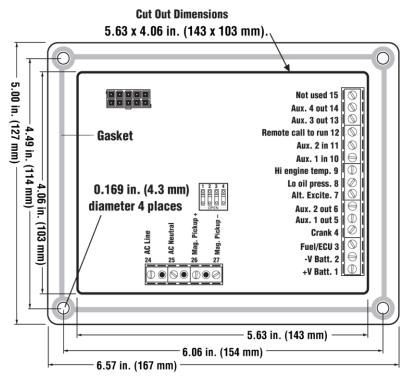
Cut a 5.63 x 4.06 in. (143 x 103mm) mounting hole, and drill four 0.169 in. (4.3mm) diameter holes for the mounting screws.
