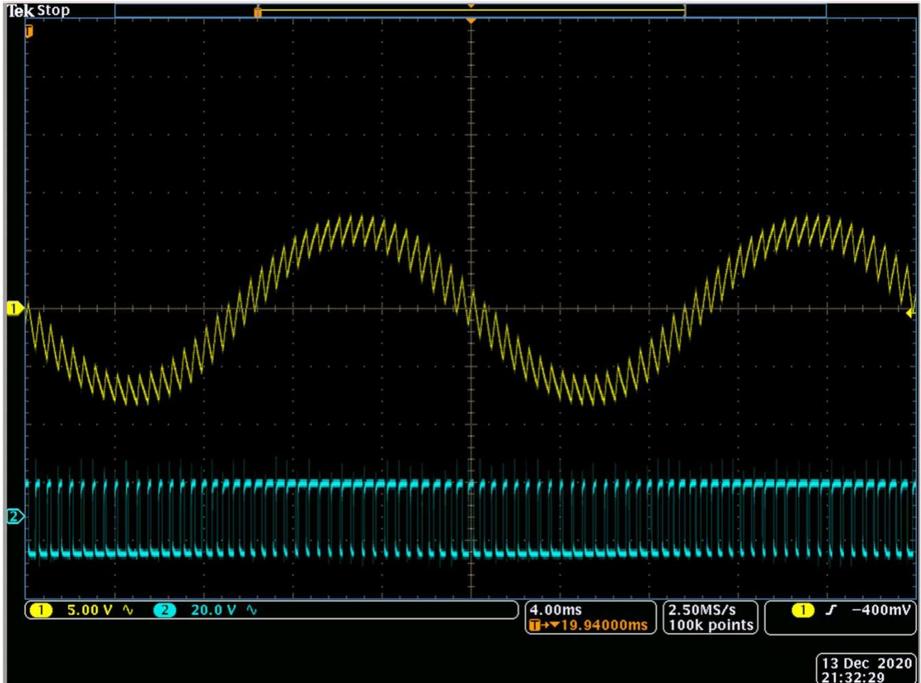
Depiction of 2 kHz PWM waveform using sinusoidal Dither (30% amplitude @ 50 Hz frequency). Lower waveform is voltage of base PWM, upper waveform is an extracted representation of the Dither signal captured using a low pass filter.
