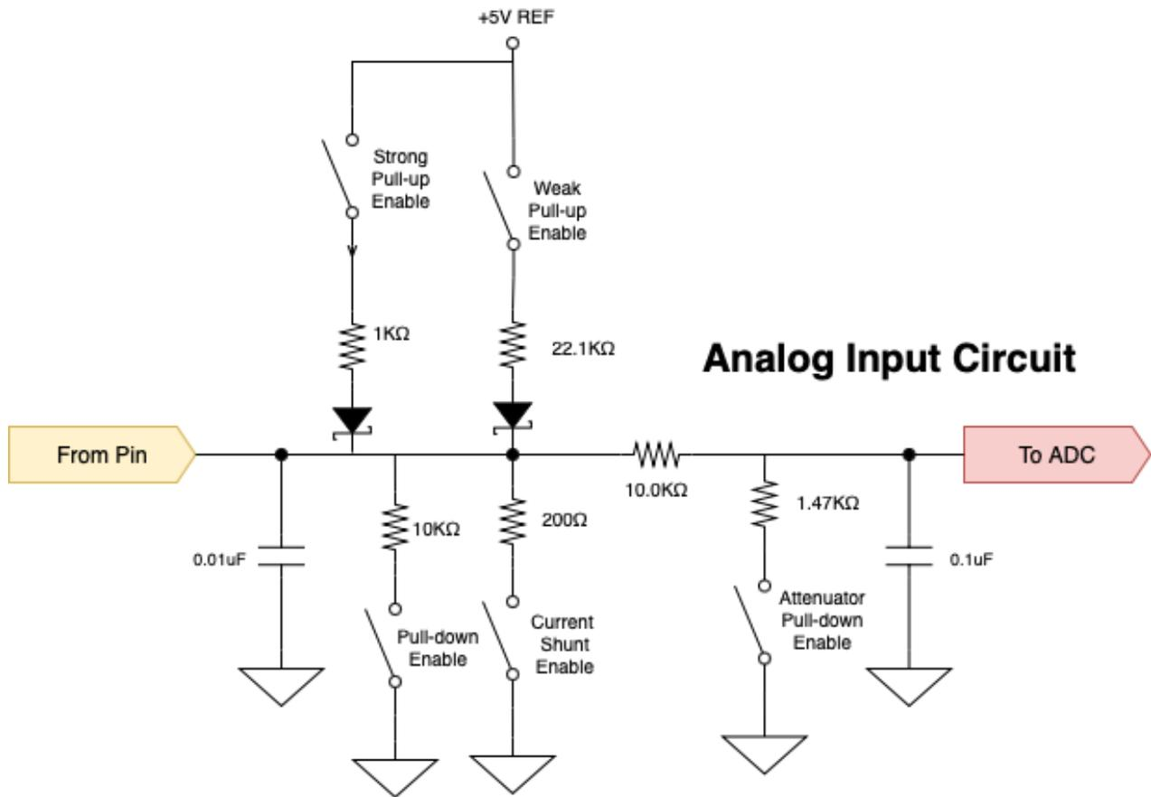
Below is a representation of the frequency input circuit and it depicts the various pull-ups and pull-downs that allow for various different operational modes required for interfacing different input devices.
