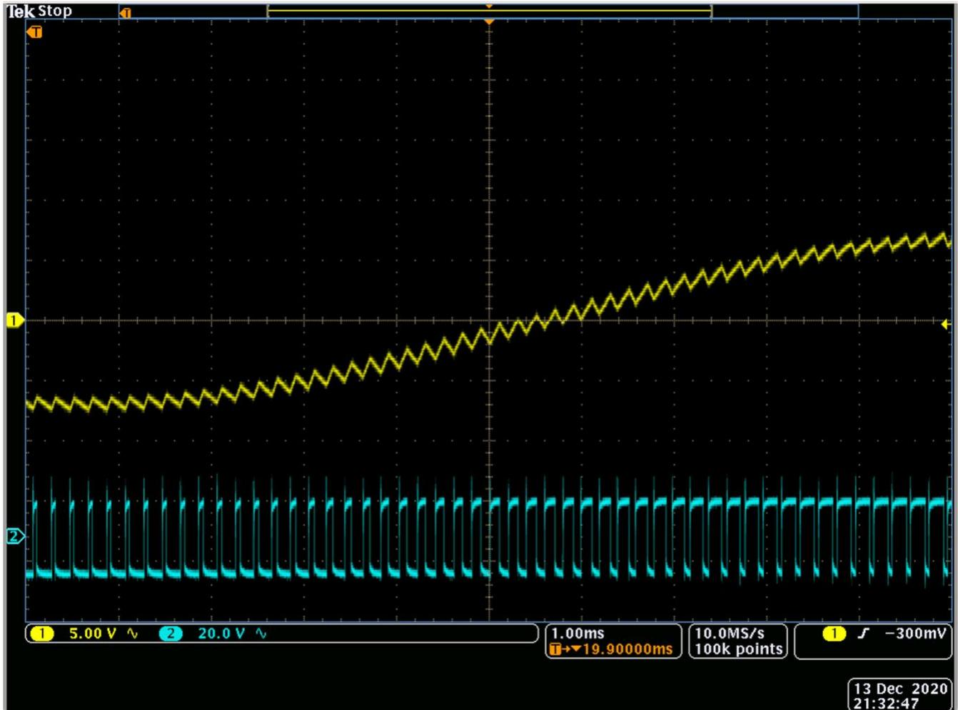
Depiction of 5 kHz PWM waveform using sinusoidal Dither (30% amplitude @ 250 Hz). Lower waveform is voltage of base PWM, upper waveform is an extracted representation of the Dither signal captured using a low pass filter. Note how this clearly depicts the Dither waveform modulating the PWM duty cycle of the base PWM waveform.
