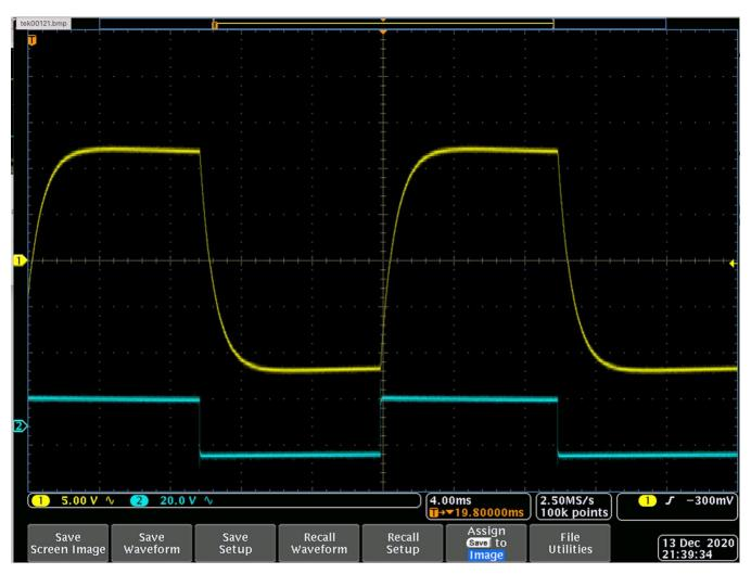
Depiction of 50 Hz PWM using no Dither. Lower waveform is voltage, upper waveform is the signal passed through a low pass filter (note no Dither present).
