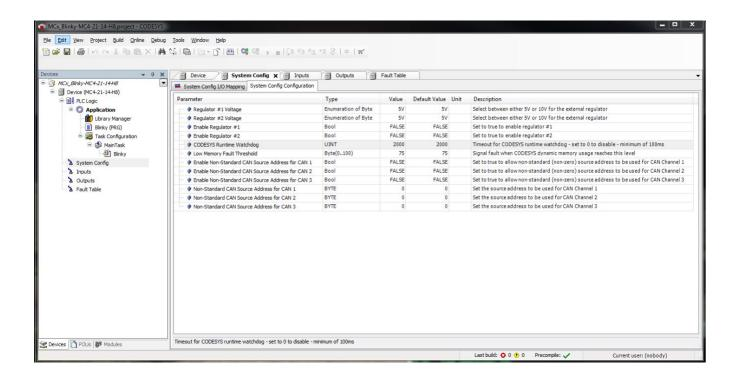
a watchdog that monitors the specific task. The time is user configurable via the Task Configuration/MainTask tab – see the screen below:
