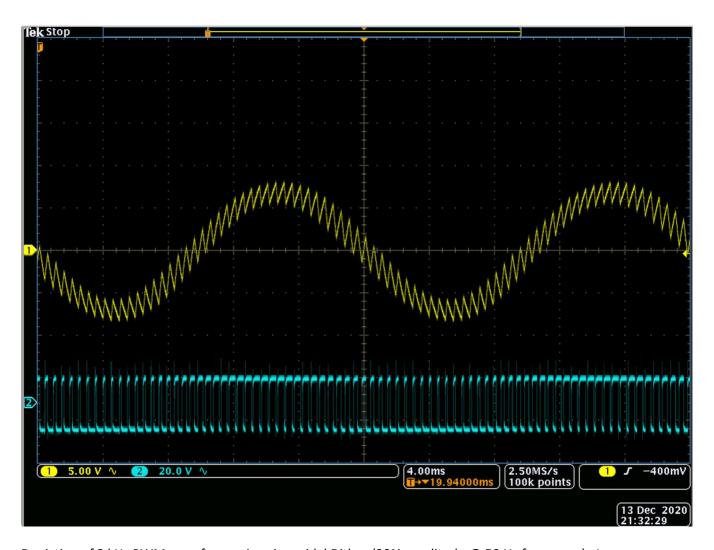
Depiction of 2 kHz PWM waveform using sinusoidal Dither (30% amplitude @ 50 Hz frequency). Lower waveform is voltage of base PWM, upper waveform is an extracted representation of the Dither signal captured using a low pass filter.
