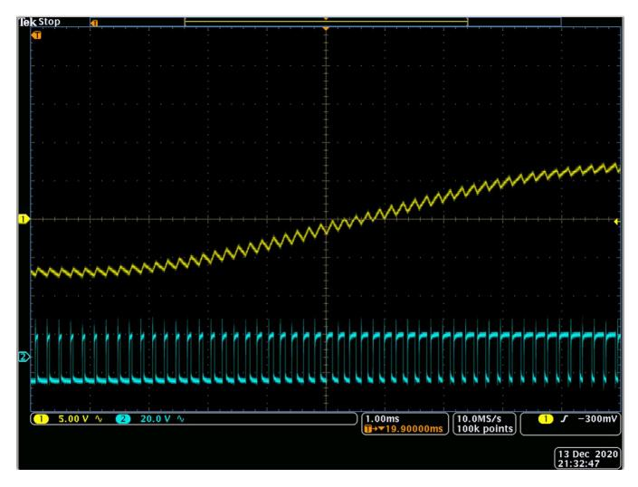
Depiction of 5 kHz PWM waveform using sinusoidal Dither (30% amplitude @ 250 Hz). Lower waveform is voltage of base PWM, upper waveform is an extracted representation of the Dither signal captured using a low pass filter. Note how this clearly depicts the Dither waveform modulating the PWM duty cycle of the base PWM waveform.
