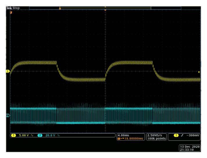
Depiction of 5 kHz PWM waveform using square wave Dither (30% amplitude @ 50 Hz). Lower waveform is voltage of base PWM, upper waveform is an extracted representation of the Dither signal captured using a low pass filter.
