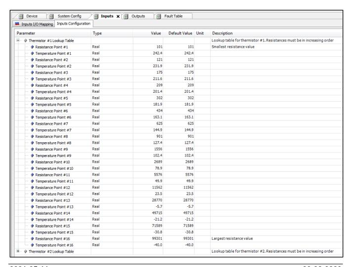
We use  $22k\Omega$  pullup resistors in this mode (thermistor 1) and therefore recommend that you use resistances in the range of  $500\Omega$  and  $100k\Omega$  for optimal performance. Additionally, a second resistive mode can be used (thermistor 2). We use a  $1k\Omega$  pullup resistor in this mode and this is best selected when resistances range between  $10\Omega$  and  $500\Omega$ .
