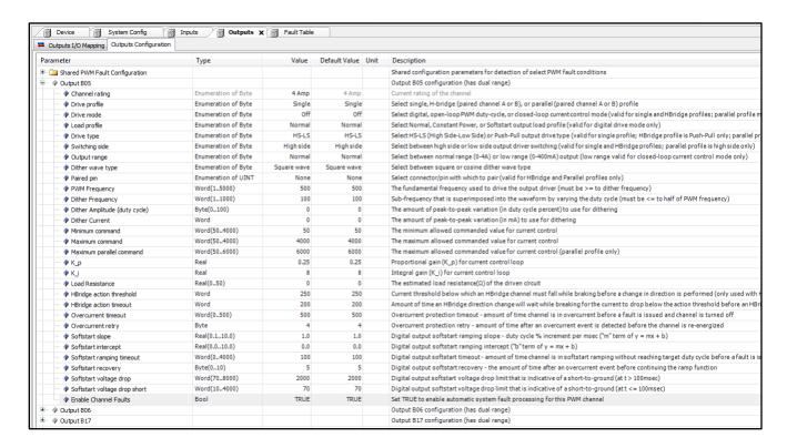
The **Outputs Configuration** tab allows the selection of the output channel's Drive Profile, Drive Mode, Load Profile (for Digital mode only), Drive Type, Switching Side, and Output Range (if dual range capable). Additional configuration settings include PWM Frequency and Dither values, Minimum/Maximum Command limits and PI control loop tuning parameters for current control, Overcurrent Timeout and Retry values, and Digital mode Softstart parameter definitions.
