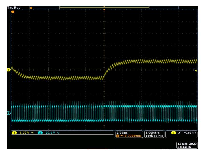
Depiction of 5 kHz PWM waveform using square wave Dither (30% amplitude @ 50 Hz). Lower waveform is voltage of base PWM, upper waveform is an extracted representation of the Dither signal captured using a low pass filter. Note how this clearly depicts the Dither waveform modulating the PWM duty cycle of the base PWM waveform.
