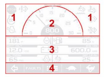
1. Alert and Warning Icon area: Up to eight symbols can be shown at one time in the icon area to represent warnings, Tier 4 status and service indicators. The most important symbol will be shown in the upper left area. The following symbols can be shown in this area:
