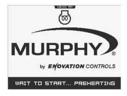
The PV380 will skip the Wait to Start (WTS) screen if the ECU stops transmitting the wait to start message or if the engine speed is >500 RPM. If the ECU never transmits the wait to start message, the splash screen is displayed for three seconds after key on, then the main gauge screen is shown.
