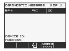
Press the  $\ \ \, \ \ \,$  and  $\ \ \, \ \ \,$  to scroll through additional messages if any are present. Each saved code shows the SPN (Suspect Parameter Number), FMI (Failure Mode
