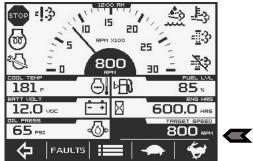
**NOTE**: Target Speed gauge appears for 5 seconds when the user throttles the engine (see arrow above)
