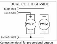
Connection detail for proportional outputs using H1/H2 and G1/G2 and J1/J2
