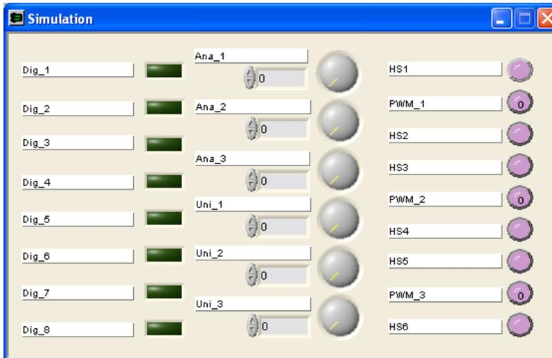
A useful facility for debugging your DVC5/7/10 application without physically being on the target machine is the application simulator. Using this facility much of your application code can be debugged prior to actually installing the controller and the application on the target machine.
