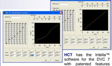
that allow the user to change the shape of the output curve relative to the input signal. This allows for optimization and accurate control of hydraulic devices that do not have very linear operating characteristics.
