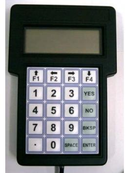
batteries and a moisture and oil proof keypad. Backlighting provides for easy reading of the display.
