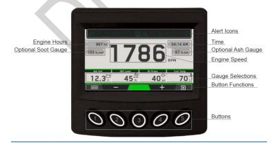
The Home screen displays Engine Hours, Time, RPM/Speed and up to 12 gauges, chosen from 62 <u>available</u> parameters.
