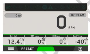
Once you press the PRESET button, the preset speed options will appear as shown in the following image. The preset speed allows the user to quickly control engine speed to a preconfigured target speed. The type of the target speed illustrated below will depend on the Target RPM Type setting in the menu. Available options are RPM or Percentage.
